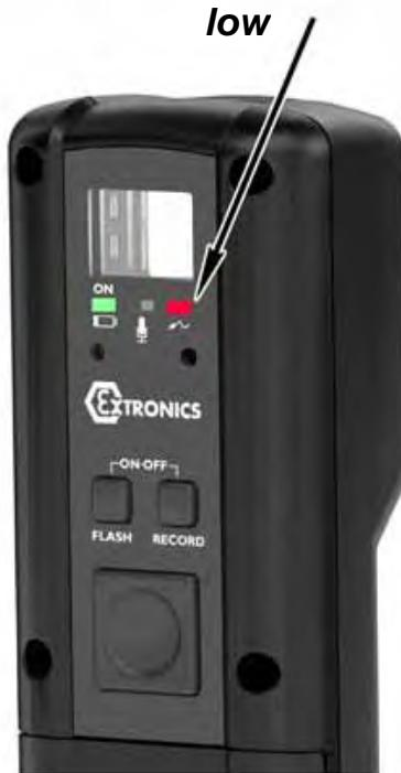
To take a picture move your eye to the view finder and position the camera so that you can see what it is you would like to take a picture of, the point of interest should be at least 30cm from the lens. The reticule can be used to frame the image you want to capture. Note that the actual picture is about 15% larger either side of the actual viewfinder image.
