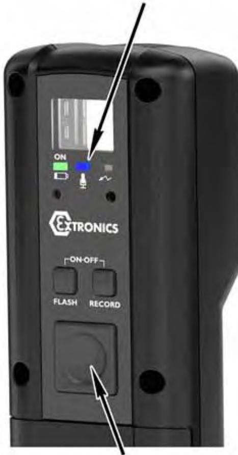
***Press and HOLD trigger button, WAIT until blue LED begins to flash, then record audio and release trigger button when finished***
