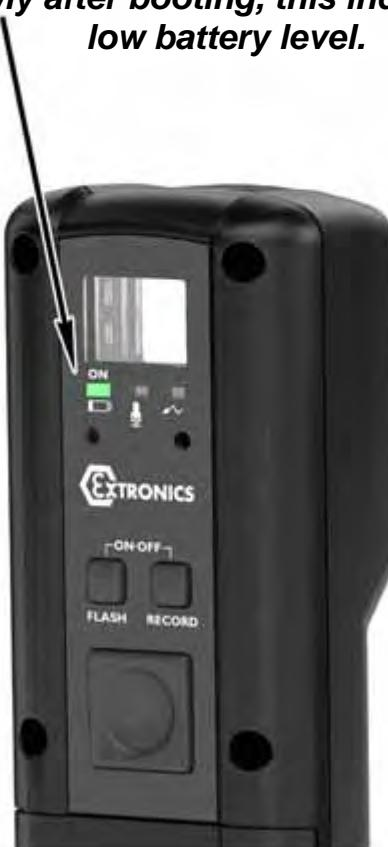
The diagrams above show how to power on the iCAM501U. The same procedure is required to turn the iCAM501U off. Once it is turned off no LED's should be lit.
