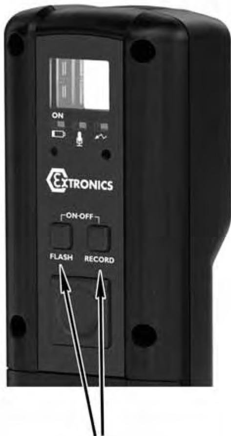
**Press and hold the “FLASH” and “RECORD” buttons simultaneously until the “ON” LED starts to flash green.**
