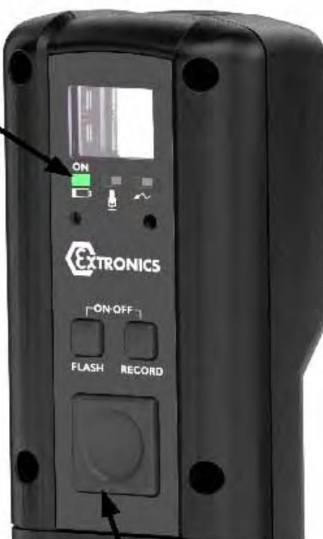
***Press and hold trigger button until green LED starts flashing rapidly, wait for green LED to stop flashing before moving***
