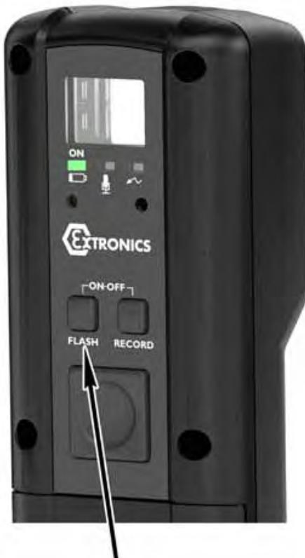
**Press the “FLASH” button to enable the flash feature of the camera.**
