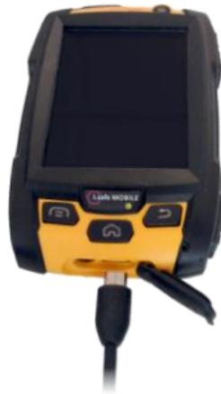
Connect the plug with the socket of the Power Supply.
