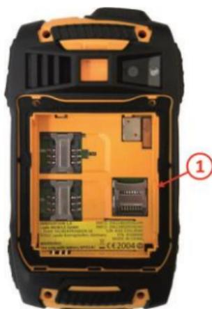
Open the Micro-SD card holder, and insert the Micro-SD card into the slot, then close the Micro-SD card holder.
