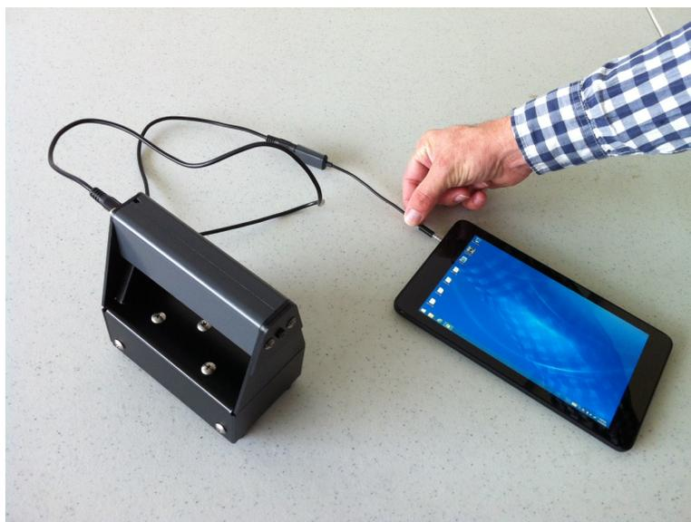
4. Flip the toggle switch on the base of the IE test head to activate the unit. When the green light is illuminated, the IE test head is powered up and ready to collect data.
