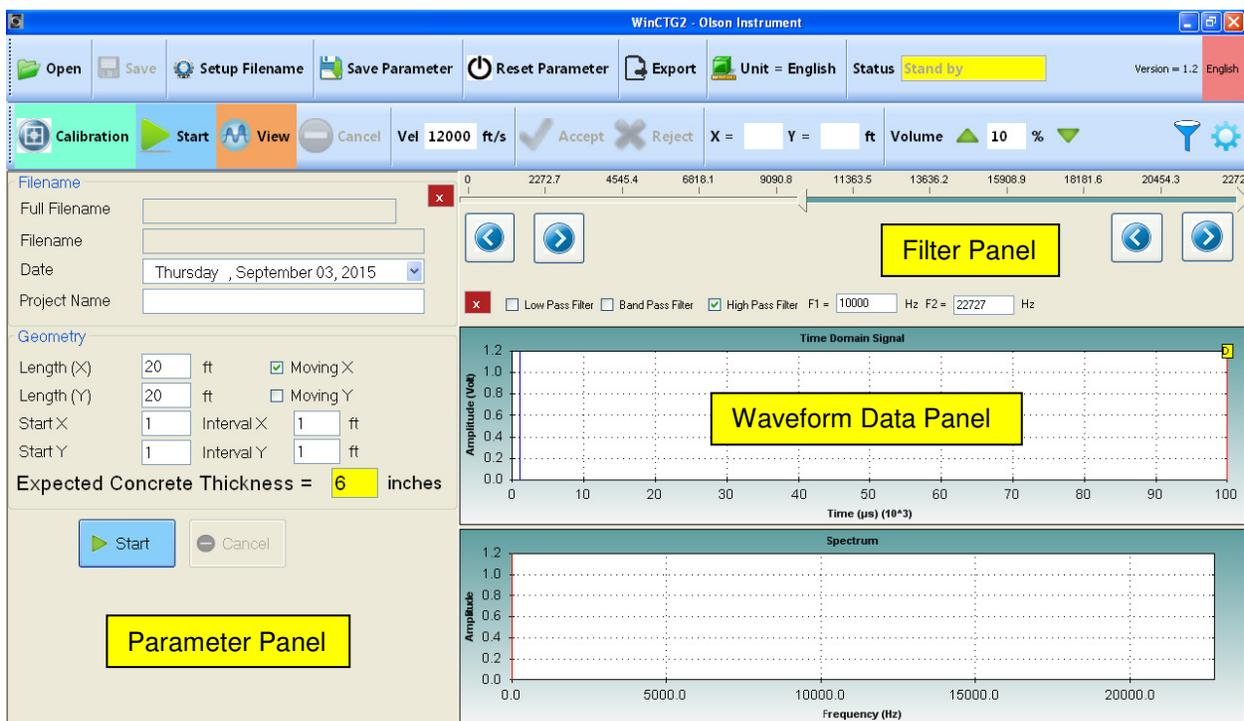
Figure 1 – WinCTG2 Layout for IE Test Results
