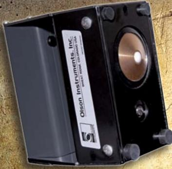
The **CTG-2** is a hand-held, battery powered, nondestructive system for measuring the thickness and integrity of concrete slabs, pavements, tunnel linings, walls and other plate-like structures using the Impact Echo principle.
