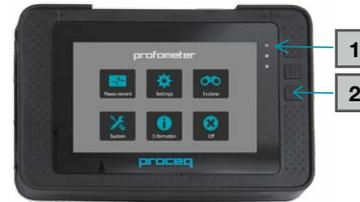
Figure 1: Main menu, leds, buttons
