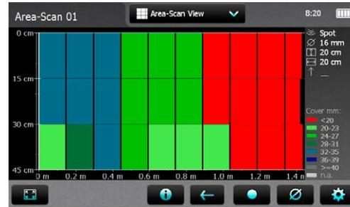
**Figure 26:** Area-Scan View (X- and Y-axis with different scale)
