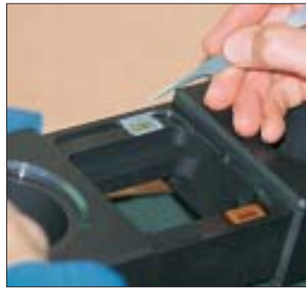
Bonding strain gauges
